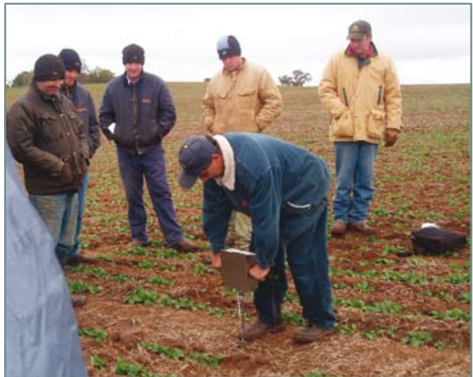
Measuring soil strength using a penetrometer at the Bobbara Station Field Day.
