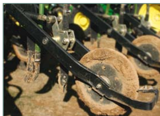
The seeding depth of each tine is controlled by the press wheel attached to it in the Conservapak parallelogram design.
