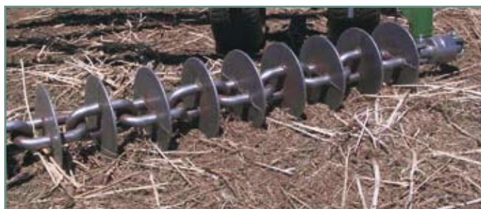
A disc chain can be used to mulch stubbles to increase the speed of breakdown and improve residue flow through seeding equipment.
