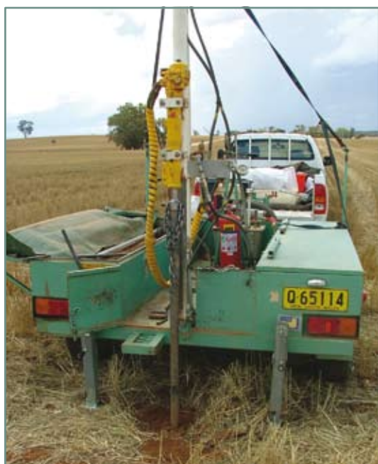
Taking soil cores to a depth of 60 cm to measure soil moisture and soil nutrient levels after harvest.
