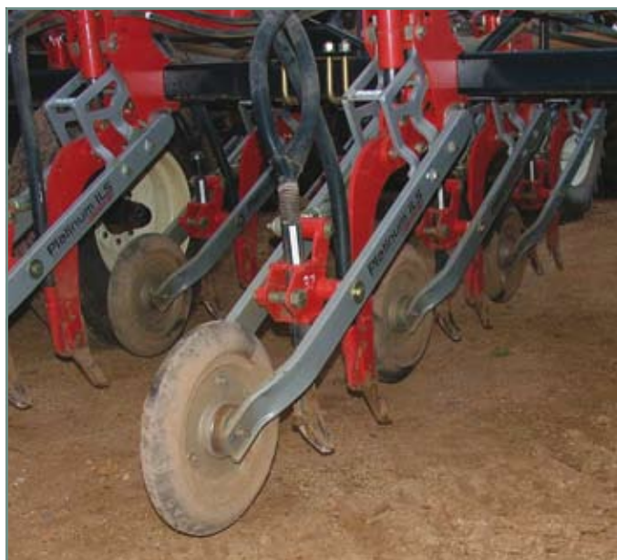
The Conserva Pak tine and press wheel assembly has a parallelogram design so the seeding depth of each tine is controlled by the press wheel.
