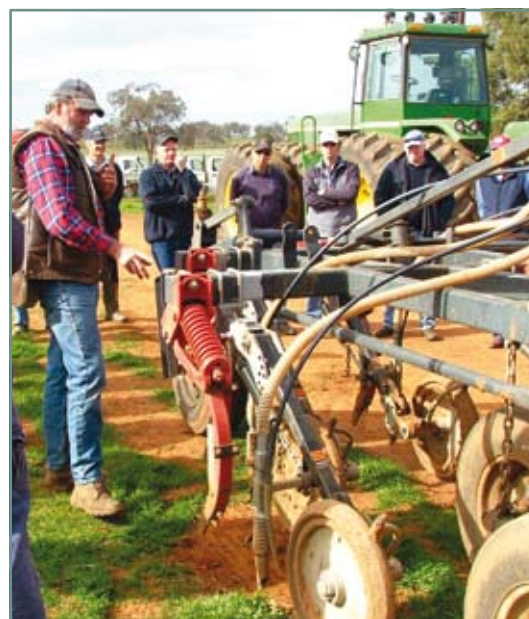
Derek Ingold explains to field day participants how the Knuckkeys tine and press wheel assembly operates to maintain uniform seeding depth.
