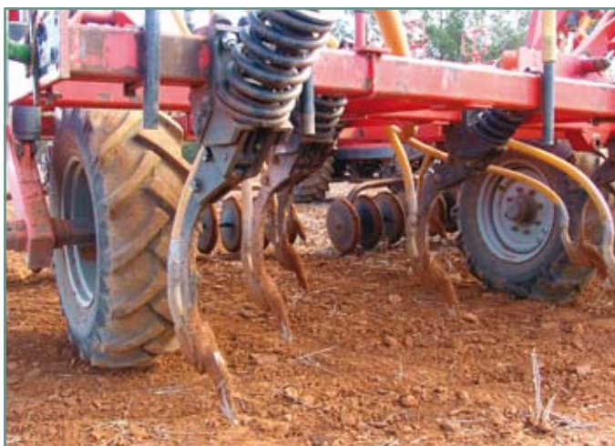
The Horwood Bagshaw airseeder used at Mukoora is set on 262 mm row space and is open to optimise trash flow at sowing.
